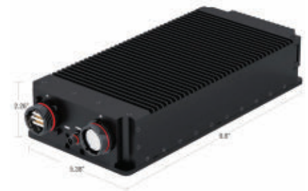
The General Micro Systems Peacock III S1202-XVE is a rugged, low profile video server.
